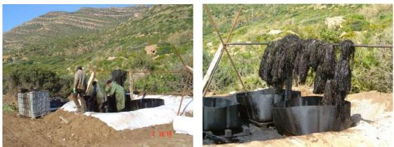
Re-use equipment, e.g. draining of Pom Pom on site for re-use (Source: Le Floch Depollution)
